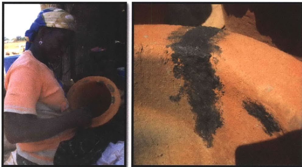
Figure 4-24: Left: Potter Patching a Filter, Right: Example of Dried Filter Patch
