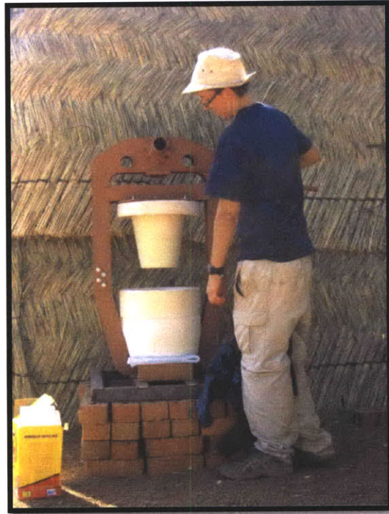
Figure 4-13: Portable Press and Nylon Male and Female Molds Used For Flower Pot Filters
