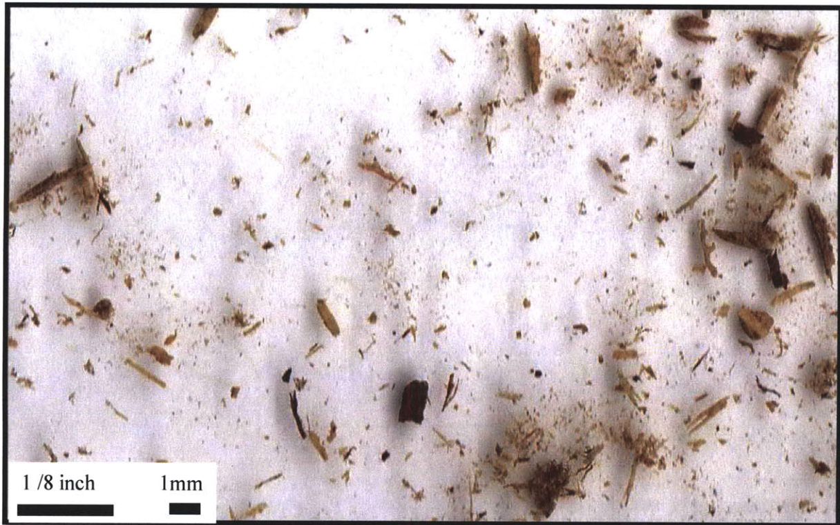
Figure 5-6: Scanned Image of Sawdust through Hammermill Fine Chute and 1mm x 1mm Sieve
