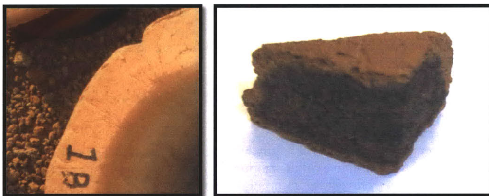
Figure 4-35: Left: Triangular Notch Cut from Filter 1B, Right: Filter Lip Piece from Filter 1B
