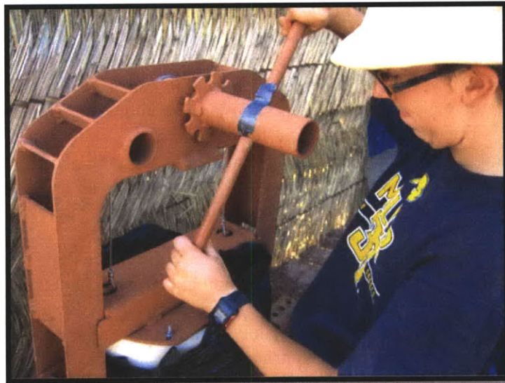
Figure 4-14: Portable Pressed Used For Flower Pot Filter, Male Mold Being Lowered
