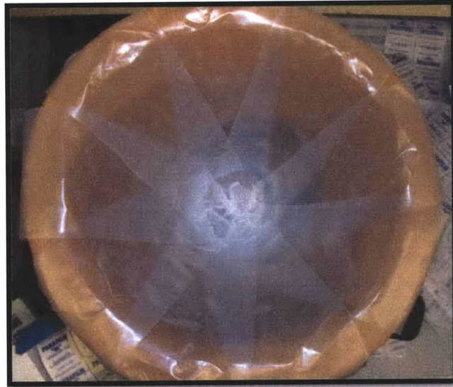
Figure 8-2: Paraboloid Filter Lined with Parafilm®
