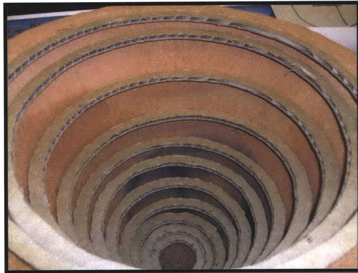
Figure 8-7: Rings of Circle Remainders Placed Inside Filter
