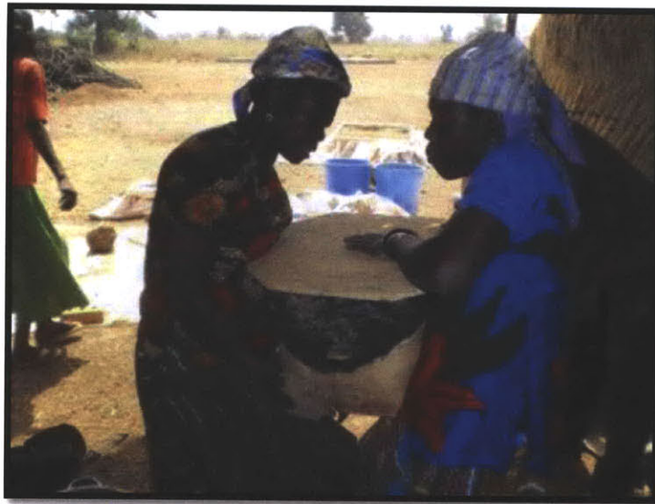
Figure 4-15: Local Potters Flipping Over Female Mold with Plywood Bat
