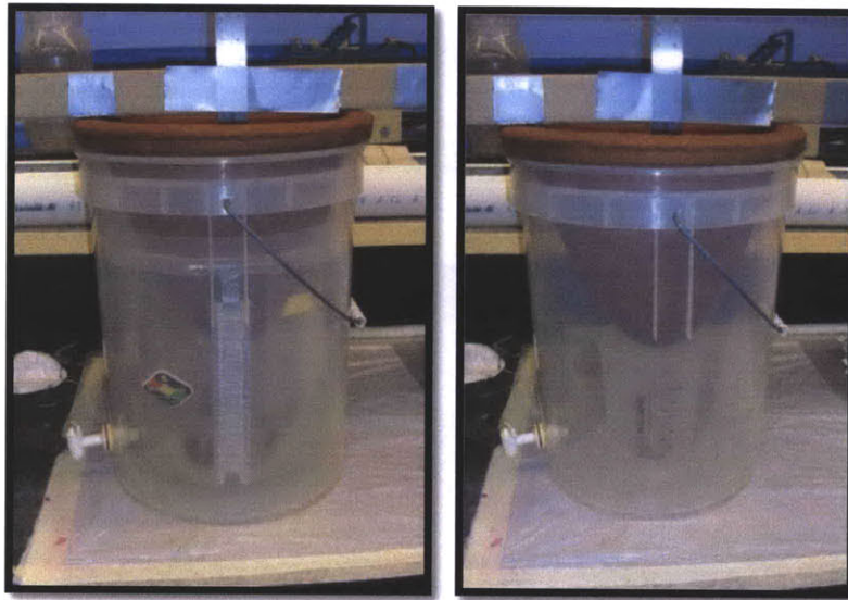
Figure 8-8: Left: Filter Set Inside Clear Bucket with Vertical Ruler Above Flowrate Container Right: Filter Set Inside Clear Bucket with Vertical Ruler Above 1L Beaker
