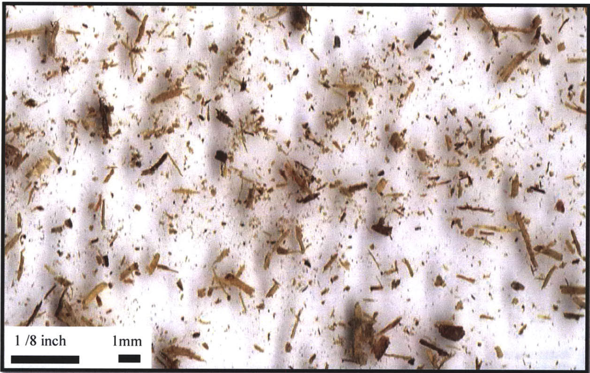
Figure 5-5: Scanned Image of Sawdust through Hammermill Fine Chute
