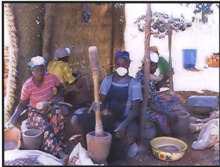
Figure 4-6: Women Pounding Clay with Large Wooden Mortar and Pestles
