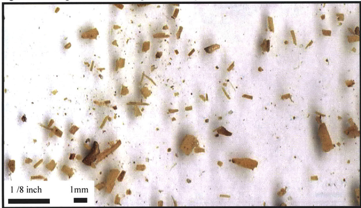
Figure 5-1: Scanned Image of Rice Husk through Hammermill Waste Chute
