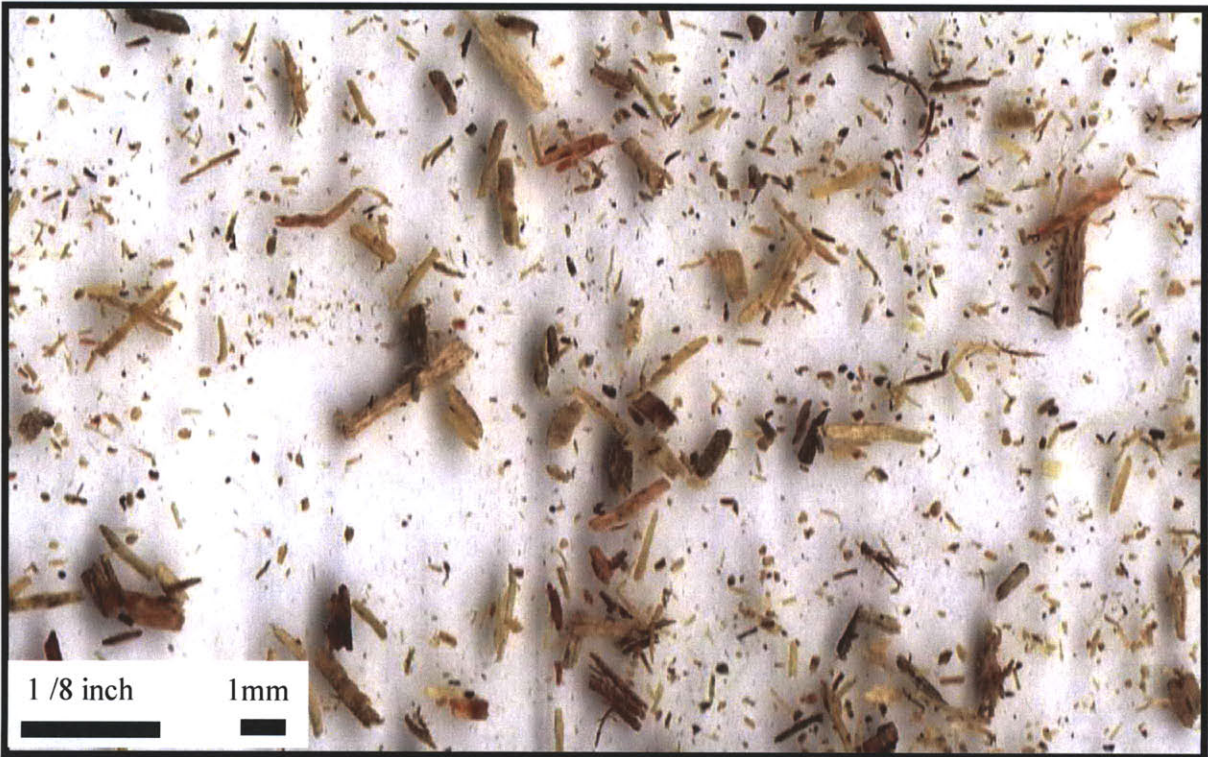
Figure 5-4: Scanned Image of Sawdust through Hammermill Waste Chute
