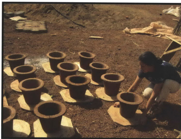
Figure 4-18: Filters Drying in Sun on Plywood Bats, Turned by MIT Team Member Leah Nation
