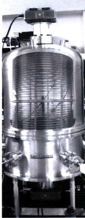
Figure 2-3: (Left) Photograph of the 10-liter DMTPC detector with an overlaid image of the dual TPC. Inside the chamber, stainless steel field shaping rings modulate the drift field. The CCD cameras are located outside the chamber on the top and bottom where they each image an amplification region. Image taken from [11].
