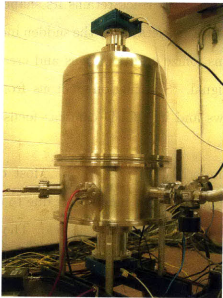
Figure 2.4: The photograph on the left shows the exterior of the chamber. The two CCDs are attached to the top and bottom of the chamber. The wires coming out of the front and left sides of the chamber are used to control the voltage of the field cage. The metal tubing to the right is used to evacuate the chamber and fill it with \text{CF}_4 gas. A seal near the middle allows the top half of the chamber to be removed. The picture on the right shows how the field cage is oriented inside the chamber. Each cylindrical TPC is composed of rings connected in series with resistors (visible along the left side of the field cage). Wire leads are connected to the TPCs as well as the meshes and the anode plate. Photo courtesy of Denis Dujmic of the DMTPC collaboration.
