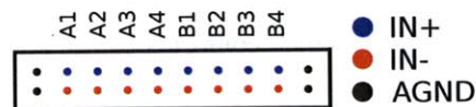
Figure 4-1: The front panel connector for the Soma Acquisition Module. AGND is connected to the amplifier analog ground.
