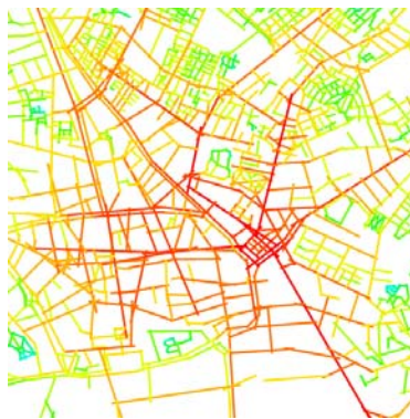
Figure 14 Space Syntax Integration analysis visualized on axial-lines of the Old Market Square area in Nottingham. Red colors refer to higher values, green colors to lower values. Source: http://www.spacesyntax.com/en/downloads/gallery/spatial-accessibility.aspx (Accessed February 24, 2010)
