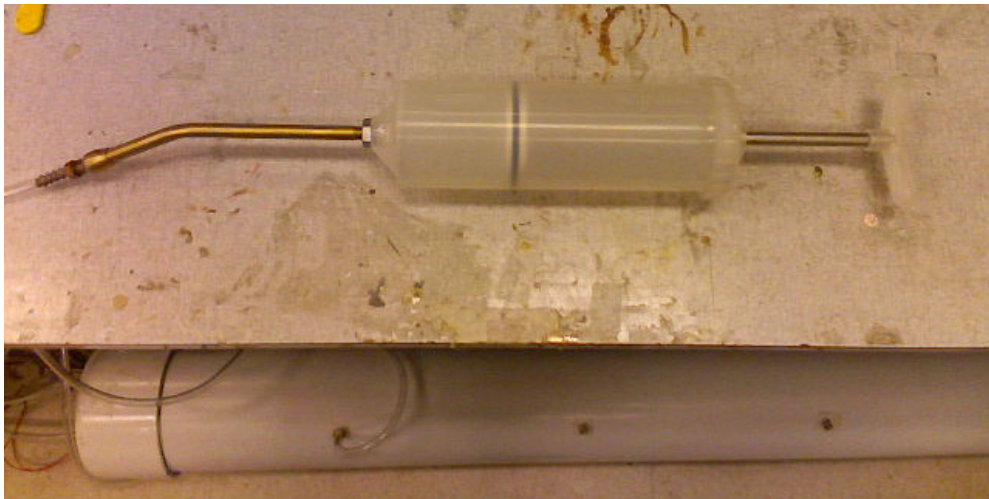
Figure 59: 600 \text{ cm}^3 syringe used for precise control of changes in internal volume (with the primary chamber visible at the bottom of the image)
