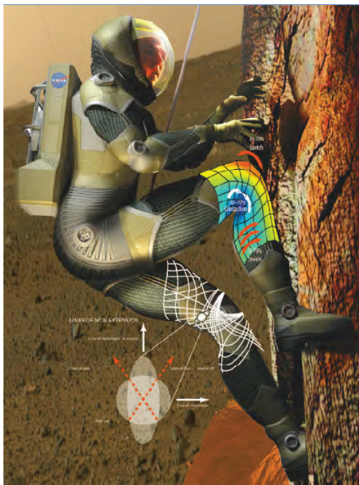
Figures 5a-b: MIT BioSuit™ concept and physical mock-up (photo credits: Dava Newman, Guillermo Trotti, Dainese, Donna Coveny)
