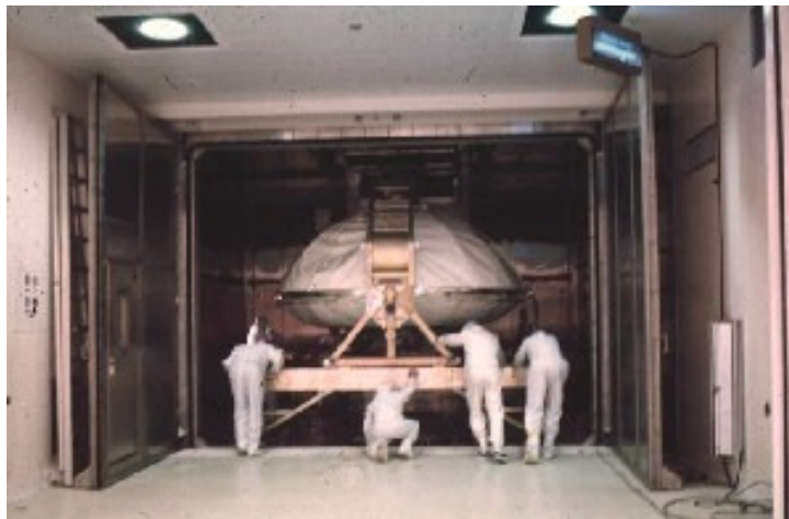
Figure 69: Dry-heat sterilization of a Viking Lander (photo credit: NASA, 2008)
