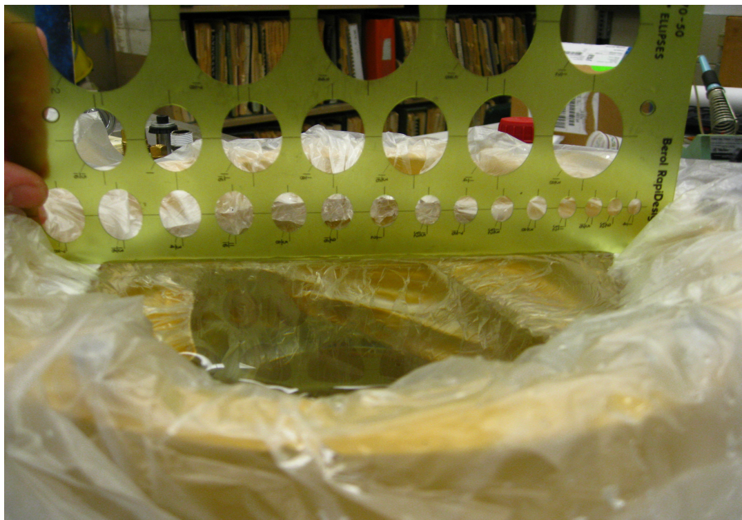
Figures 24a-c (clockwise from top left): Engineer measuring the total water required to fill the arm at 25° flexion; close-up views of the protective lining and leveling tool used to determine exact water levels at each angle
