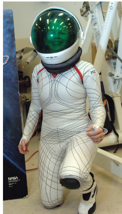
Figures 5a-b: MIT BioSuit™ concept and physical mock-up (photo credits: Dava Newman, Guillermo Trotti, Dainese, Donna Coveny)
