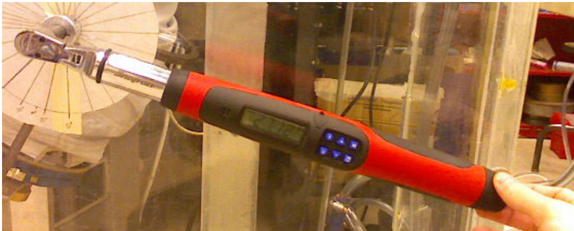
Figure 18: Electronic torque wrench configured to the EMU articulation rig
