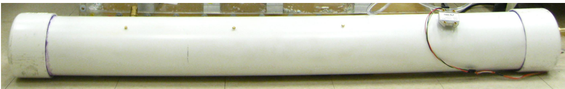
Figure 48: Primary chamber, constructed from Schedule 40 PVC pipe
