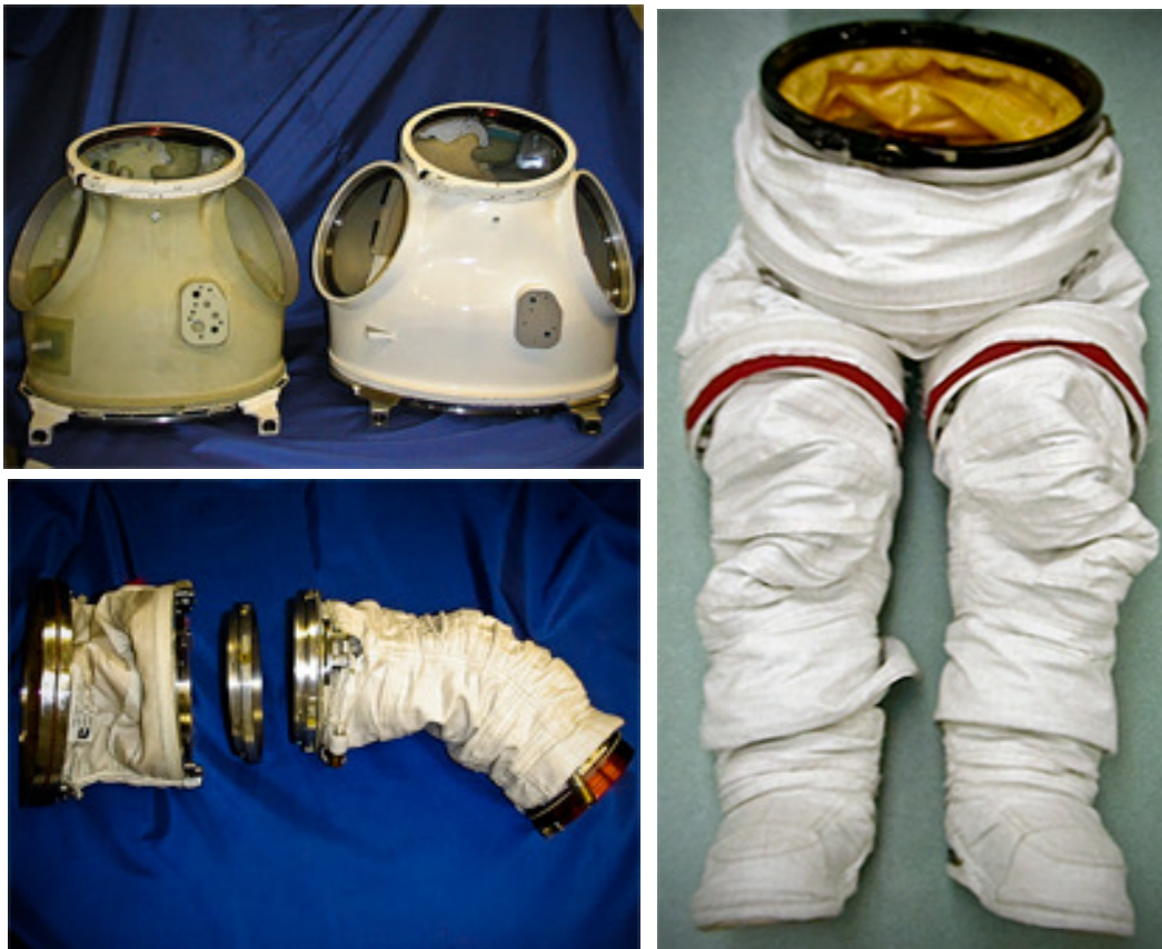
Figures 4a-c (Clockwise from Top Left): The EMU HUT, EMU waist bearing and knee joints, and EMU shoulder and elbow joints, taken from (NASA, 2008)
