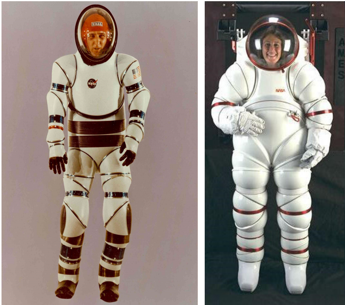
Figures 3a-b: The AX-2 suit (1968) and AX-5 suit (1988), which utilize hard joint segments separated by bearings to maintain constant volume during movement, taken from (Kozloski, 1994) (NASA, 1988)
