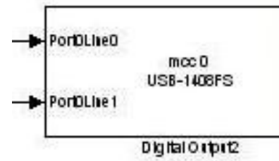
Figure 56g: USB-1408FS digital output block
