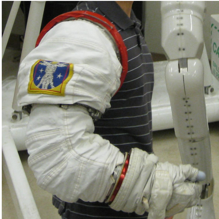
Figure 10: One of two Class III EMU arm section provided by Hamilton Sundstrand (pictured with glove attached)
