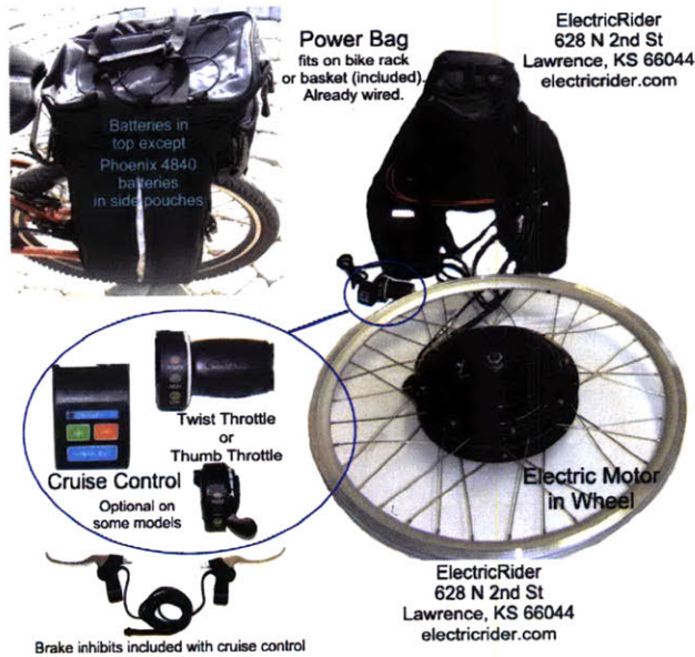
Figure 1.2: This is a good representation of the typical e-bike kit contents. In order to transform an existing bicycle into an electric bicycle, the wheel must be re-spoked with the new hub motor and the rest of the components must be mounted and wired to the frame of the bike.
