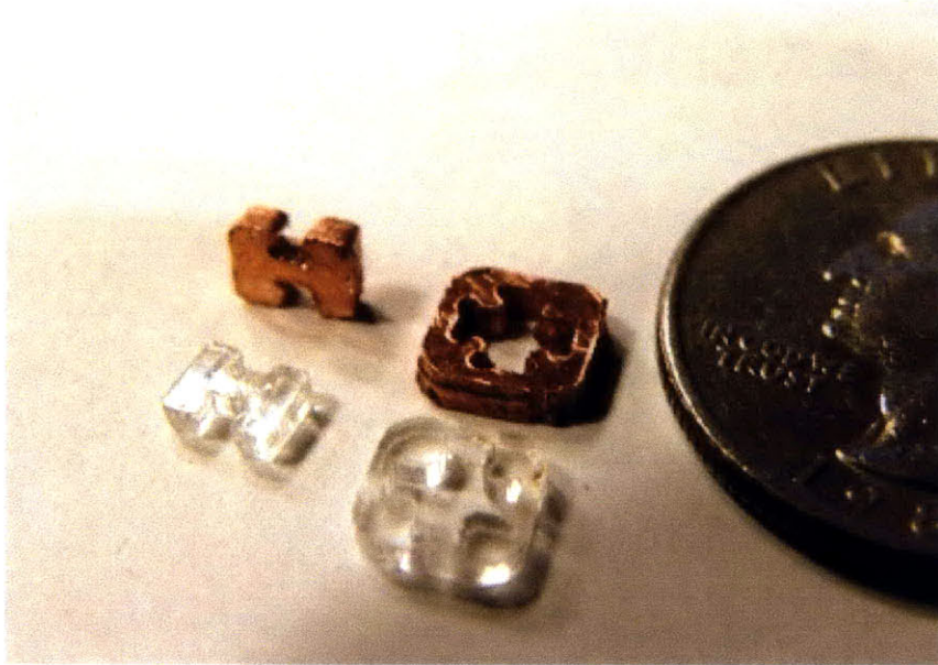
Figure 4.5b Copper and Acrylic press-fit parts
