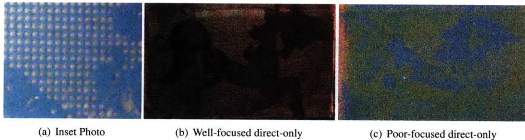
Figure 4-1: Direct-only images by Nayar et al. method for a horse-shaped object enclosed in an aquarium with diluted milk (Concentration 0.11%) (a) Inset of a captured photo with a projected high-frequency pattern (b) Direct-only image in a well-focused case (c) Direct-only image in a poor-focused case
