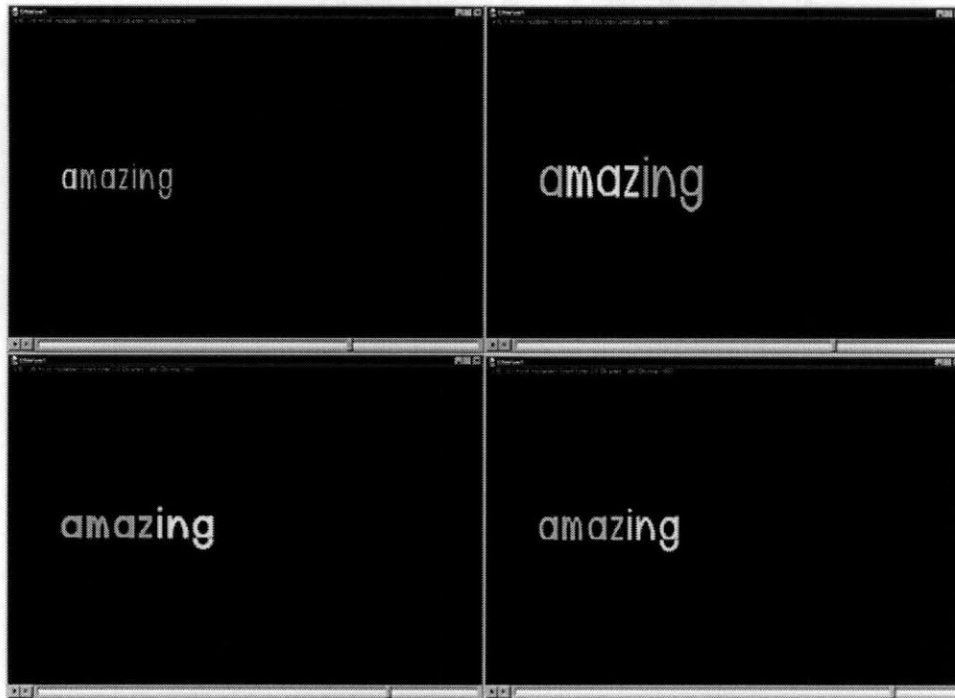
Figure 39: As a timing counter proceeds through the speech data, the syllable currently considered active is highlighted. All visual manipulations that occur are associated with the vocal transformations that occur during the vocalization of that particular syllable. Interesting visual effects may occur by freezing each syllable at the moment activity transfers to the next syllable. Prosodic Font words would then appear as collages in process.
