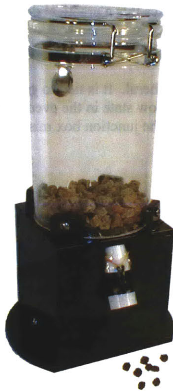
Figure 10-3: Closeup of the custom designed feeder. The top is a 4" diameter x 12" high acrylic canister. The bottom is sawed off and attached to the base with four sheetmetal screws. The screws protrude into the canister and stir the food as the rotator turns, preventing food from simply turning with the rotator.
