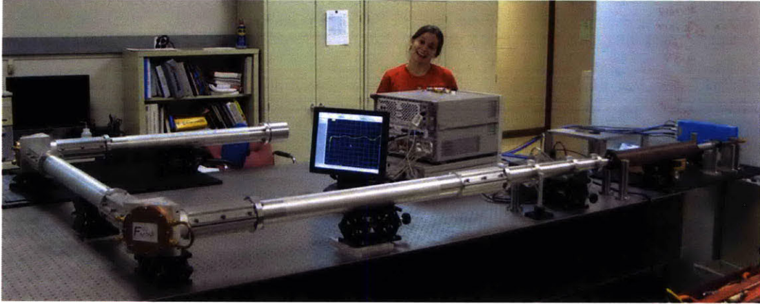
Figure 5-1: Photo of the experimental set-up for measuring the loss in a miter bend. The set-up uses three 1-m sections of straight waveguide and 2 miter bends.
