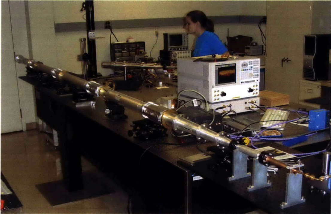
Figure 5-3: Photo showing 4 m of straight waveguide under test. The measurement of the loss due to straight sections of waveguide was used to calculate the baseline measurement and the uncertainty error of S_{3m} .
