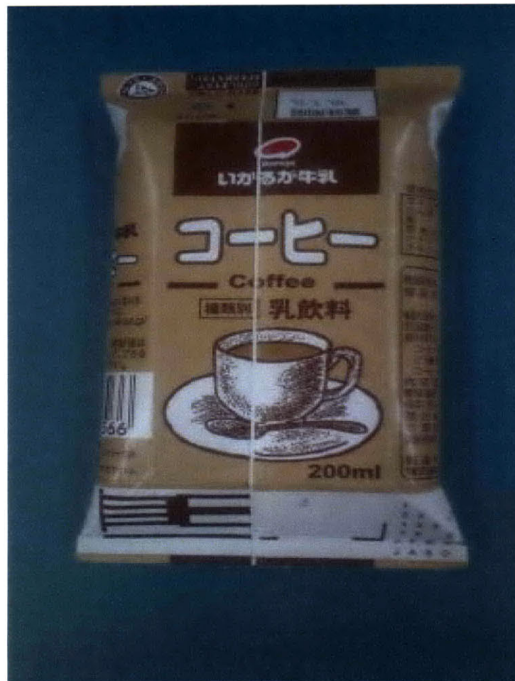
Figure 3.7 Incorrect Slitting with White Line [2]
