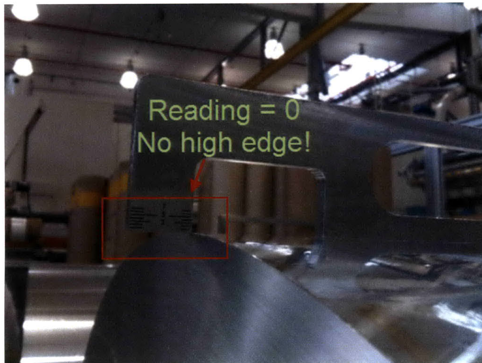
Figure 2.4: Edge Measurement of the Al Foil Roll
