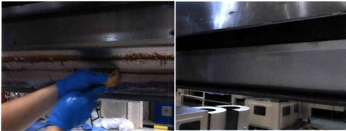
Figure 4.4: Die Cleaning for Disturbance Removal
