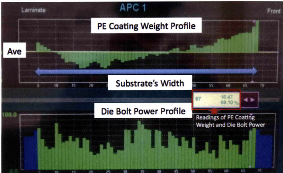
Figure 3.6: PE Coating Profile and Corresponding Die-bolt Power
