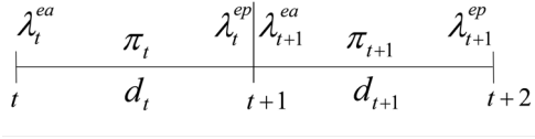
Fig. 1. \lambda_t^{ea} ( \lambda_t^{ep} ) is the exanté (ex-post) LMP for [t, t+1] , \pi_t is the retail price for [t, t+1] and it is announced at the beginning of the interval, d_t is consumption during [t, t+1] , and will be known at time t+1 .
