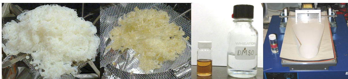
Figure 2.6. Polymer-to-membrane illustrated (from left): P(AN- r -SPA)- g -PEO polymer as precipitated into water, dried, dissolved in DMSO, and being coated onto a PAN base membrane.
