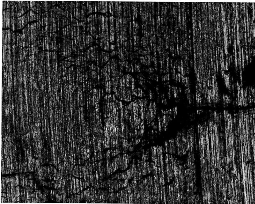
Figure 40. Crack tip region of specimen 617-CT-29 showing secondary cracks ahead of the main one
