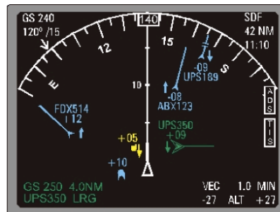
Figure 1: ADS-B Traffic Display
