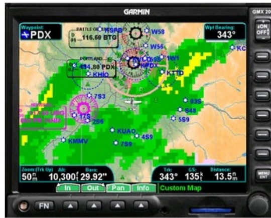
Figure 9: FIS-B Information Displayed on MFD
