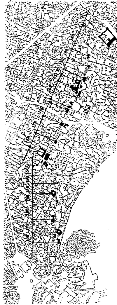
Fig. 3.13 Intervals of street intersections along the Processional Route. The average interval is 150m.
