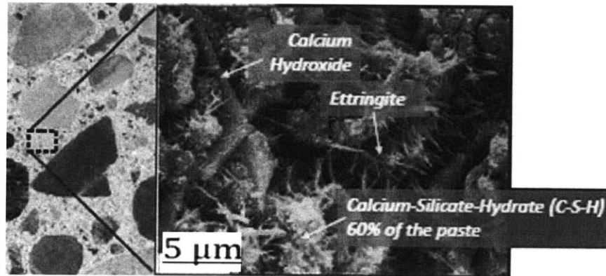
Figure 2-1: A magnified image of major cement hydration products. [Courtesy of Dr. James Beaudoin and Dr. Aalizadeh, National Research Council of Canada].
