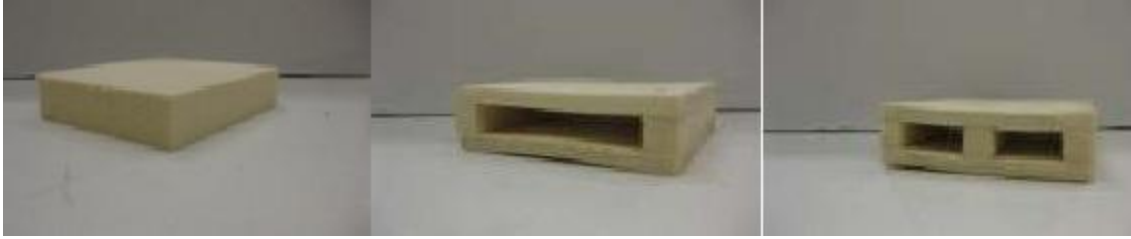
Figure 3-5 - (left) Solid block of VN600 (center) single channel (right) dual channel (4)
