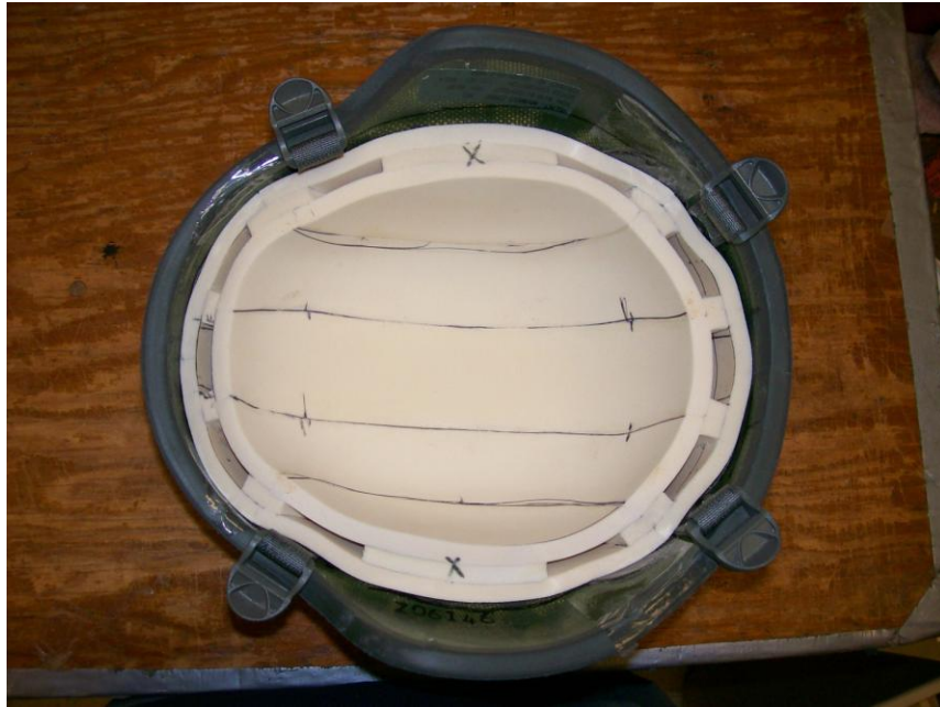
Figure 5-4 - The prototype liner installed in the ACH shell
