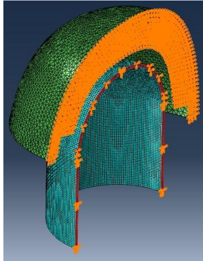
Figure 6-8 - Orange and red regions correspond to locations of symmetry boundary conditions
