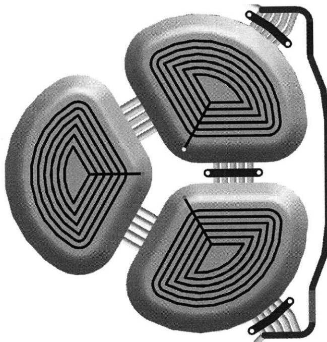
Figure 2.42. Illustration of the pass-through channel to the side of the growth chamber. Valves located in the section connectors select whether the connector or the pass-through channel are used for mixing. Since the pass-through channel does not contain a flexible membrane, long term liquid accumulation or removal from the growth chamber is reduced.
