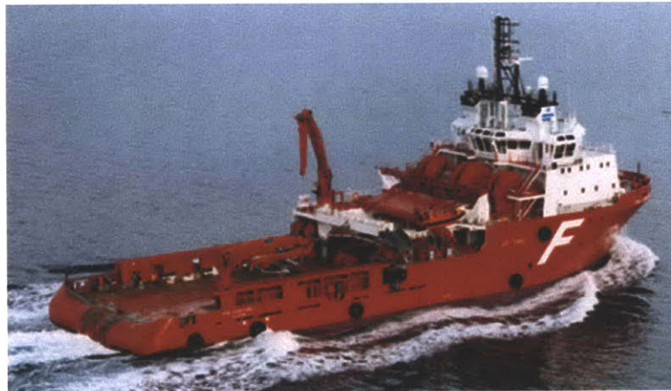
Figure 2-5: The Far Santana , a 77 meter, 203 tonne bollard pull AHTS [21].
