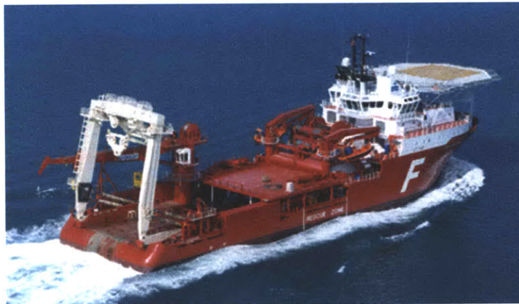
Figure 2-8: The Far Sovereign , an 85 meter, 3,631 deadweight tonne MPSV [21].
