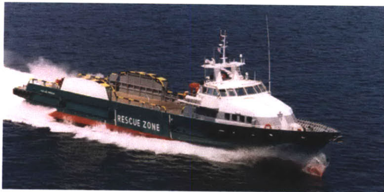
Figure 2-6: The Bourbon Express , a 50 passenger, 263 deadweight tonne FSIV [22].
