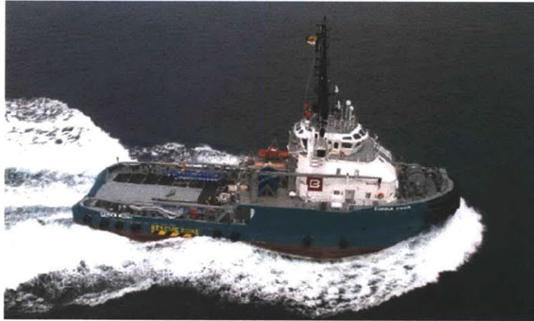
Figure 2-9: The Bourbon Rhesos , a 100 tonne bollard pull offshore tug [22].
