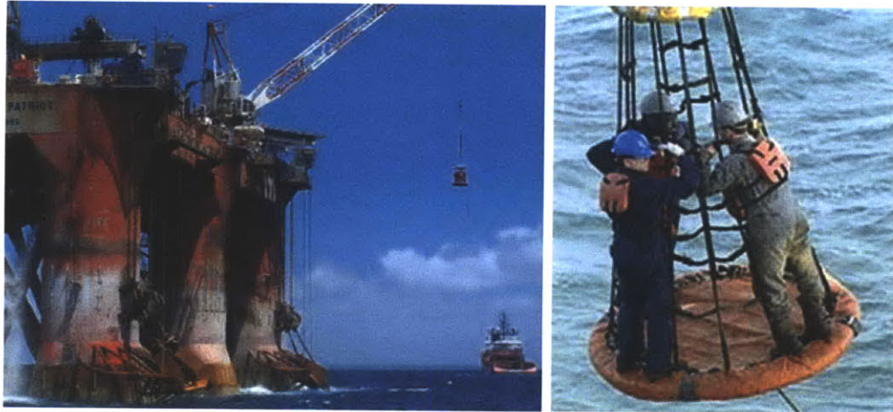
Figure 2-13: left: a crew basket hoisted from a platform [28], right: a typical crew basket [29]
