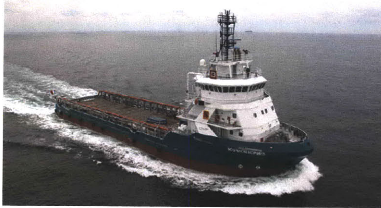
Figure 2-3: The Bourbon Hermes , a 73.20 meter, 3,230 deadweight tonne PSV [22].
