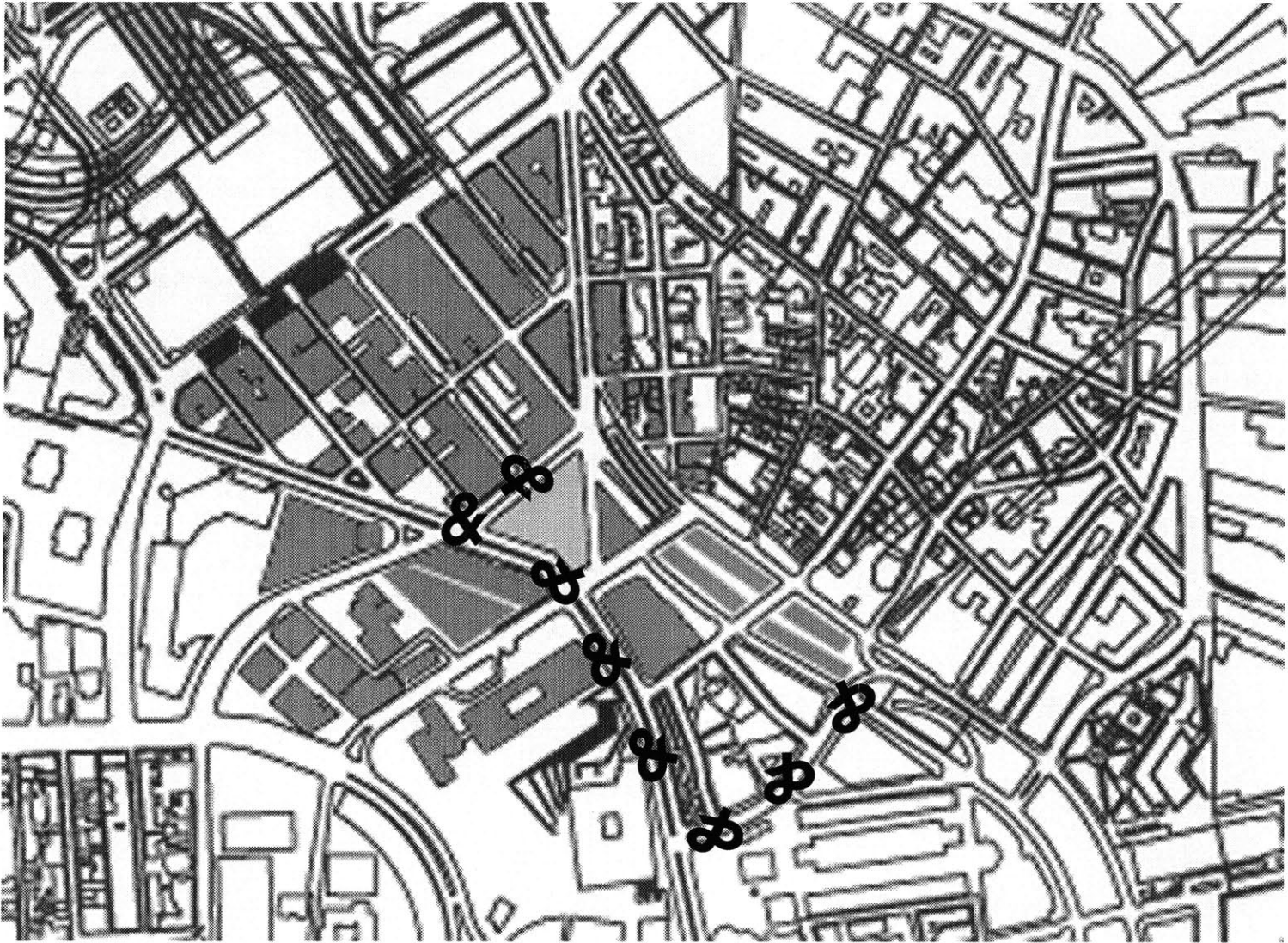
Truck Access to site from the underground artery and I-93
