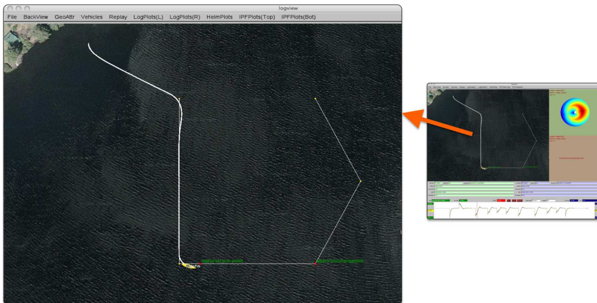
Figure 40: The OpArea panel of the alogview tool: Vehicle position(s) for a given point in time are rendered along with vehicle trajectory history and certain geometric visual artifacts such as points, polygons and line segments that may have been posted by the helm or another MOOS process. The image in this figure can be replicated exactly by launching alogview on the alpha.alog file from the Alpha mission distributed with the MOOS-IvP source code, launched with the --nowtime=144 command line option.
