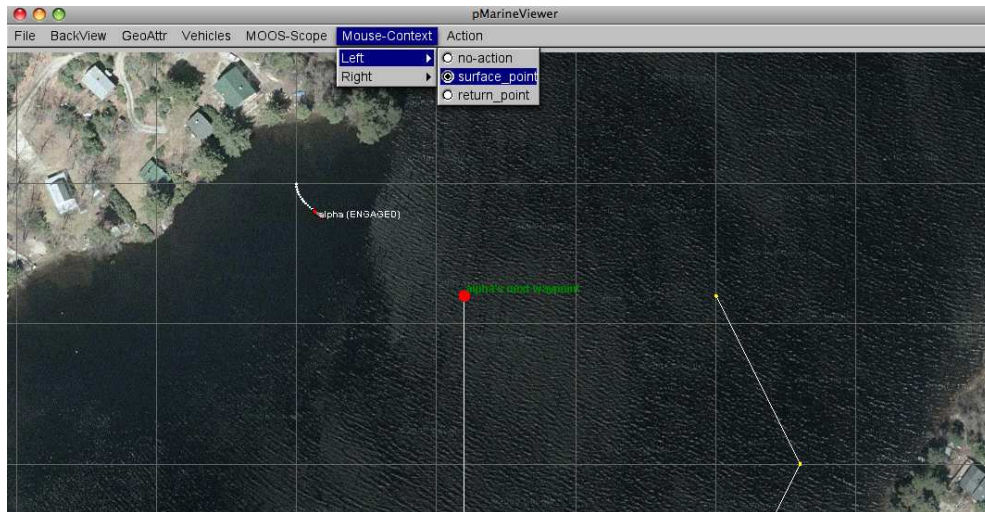
Figure 8: The Mouse-Context menu: Keywords selected from this menu will determine which groups of MOOS variables will be poked to the MOOSDB on left or mouse clicks. The variable values may have information embedded indicating the position of the mouse in the operation area at the time of the click.
