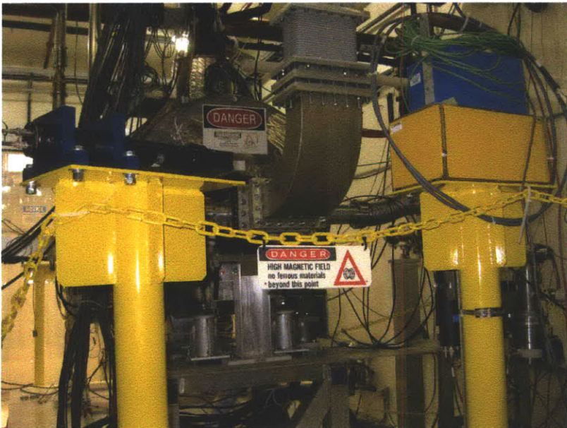
Figure 8-4: Front view of solenoid and RF power feed in MTA. For orientation, the beamline comes from the back right in this picture.
