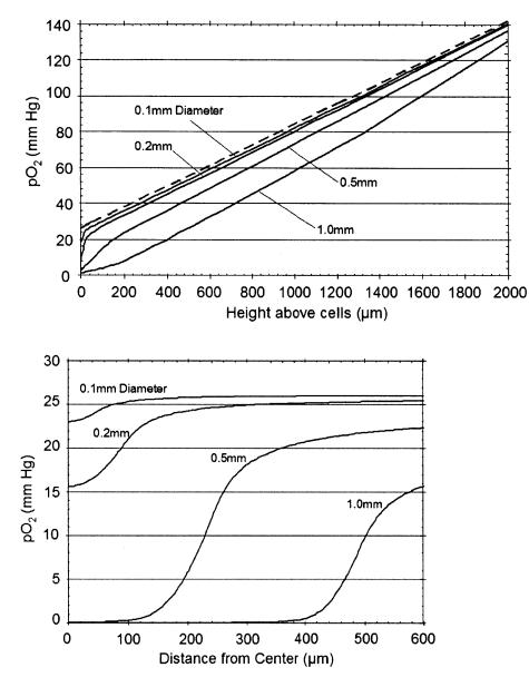
Figure D-2. Numerical simulations of oxygen sensors within oxygen gradient. (Top) Numerical simulation of  $pO_2$  measurements by probes 0.1, 0.2, 0.5, and 1.0 mm in diameter as a function of height above respiring cells in 2 mm of media. The dashed line is the calculated  $pO_2$  without any probe. (Bottom) Numerical simulation of the  $pO_2$  profile across the surface of probes of different diameters placed 20 µm above the surface of respiring cells.
