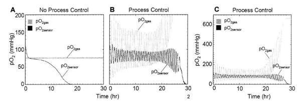
Figure D-3. Control of pO<sub>2sensor</sub> by controlling pO<sub>2gas</sub>.
