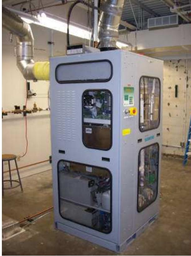
Figure 8-2: A 5 kW Siemens / Fuel Cell Technology stack used for testing.
