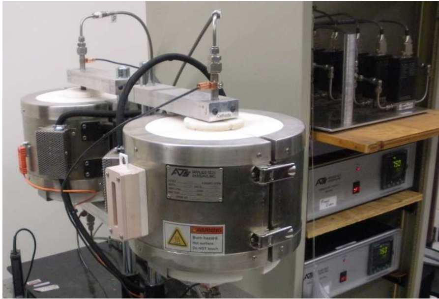
Figure 9-17: A closeup photograph of the two solid-oxide fuel cell ovens, temperature control units and mass flow controllers used in the integral diagnostics experiments.
