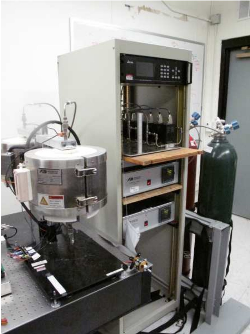
Figure 9-16: A photograph of the two solid-oxide fuel cell ovens, temperature control units and mass flow controllers used in the integral diagnostics experiments.
