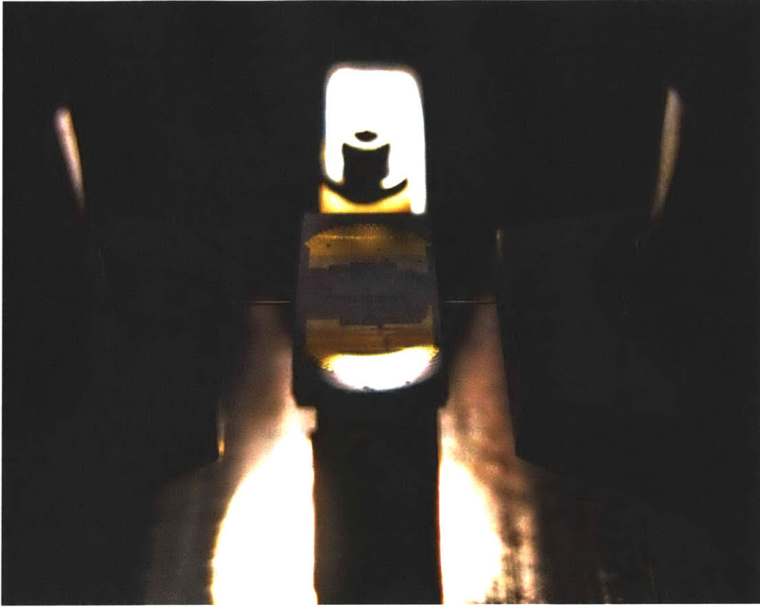
Figure 4-7 – Input and output coupling of light into the silicon waveguides using two lens-tip fibers.
