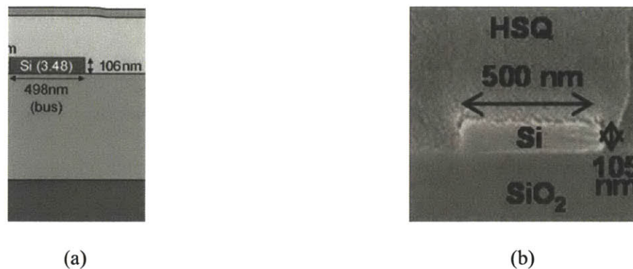
Figure 4-2 – a) Silicon waveguide structure grown on silicon substrate with \text{SiO}_2 and HSQ cladding layers[67]. b) SEM of the cross section of the chip showing the waveguide and the cladding layers[68].
