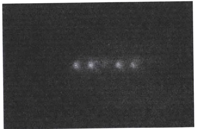
Figure 6-4: Images of trapped ions above Giants5 in a cloud state (left) and a crystallized state (right). The non-fluorescing ion is not \text{Sr}^{88} , though mass spectroscopy was not performed to verify the species.
