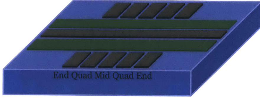
Figure 3-2: The five-wire surface-electrode trap configuration with additional DC electrodes placed on the outside of the RF so confine an ion along the three electrodes from Figure 3-1.
