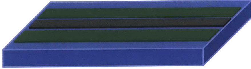
Figure 3-1: The basic configuration of electrodes for a surface-electrode trap. The green electrodes are the two RF signals and the black electrode is DC. This geometry is also consistent with the coplanar waveguide transmission line.
