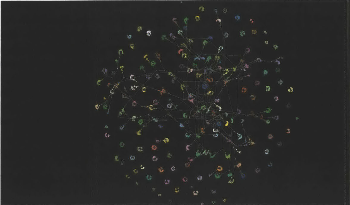
Figure 3-5: Graph embedding-based visualization of male speaker i-vectors after inter-session compensation. Points grouped close together represent the same speaker, while the visible edges between clouds also represent close proximity between two points (via the cosine distance metric). Figure taken from work done on [6, 7]; reproduced with permission from the authors.
