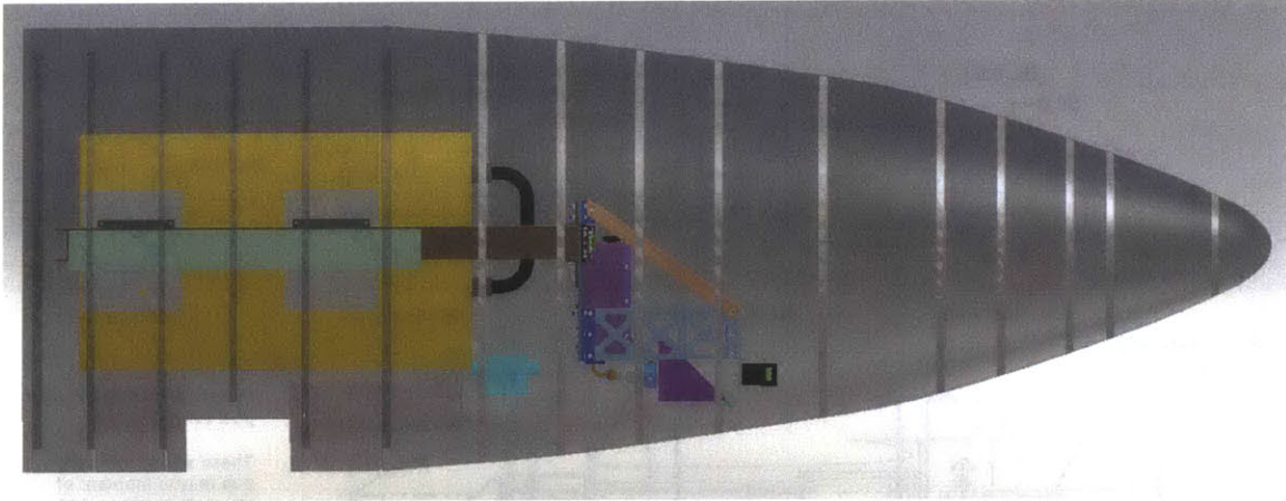
Figure 3-9: A side view of NAST-M and NAST-K in the aft wing pod of the ER-2. NAST-M can be seen in yellow and the smaller assembly mounted off of the brown support rails is NAST-K. The metal structural rings of the pod can be seen in white. [6]
