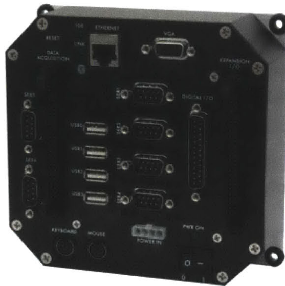
Figure 3-4: Flight computer enclosure I/O panel. [8]
