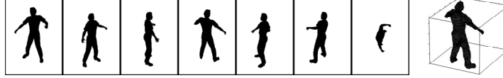
Figure 2: Examples in the model are composed of some number of silhouette views, plus their camera calibration parameters.
