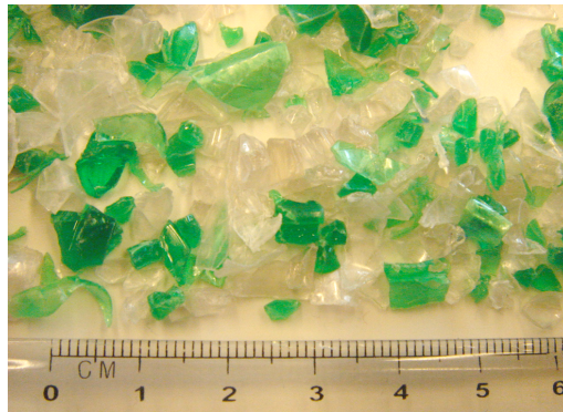
Figure 6-1: Typical PET material as prepared for magnetic roller separation, with scale in centimeters (from [75]).
