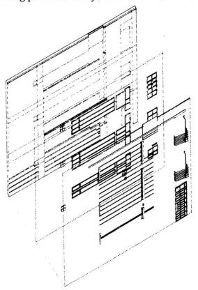
Fig:I.1, Exploded axonometric depicting the thin layers of the building's facade.
