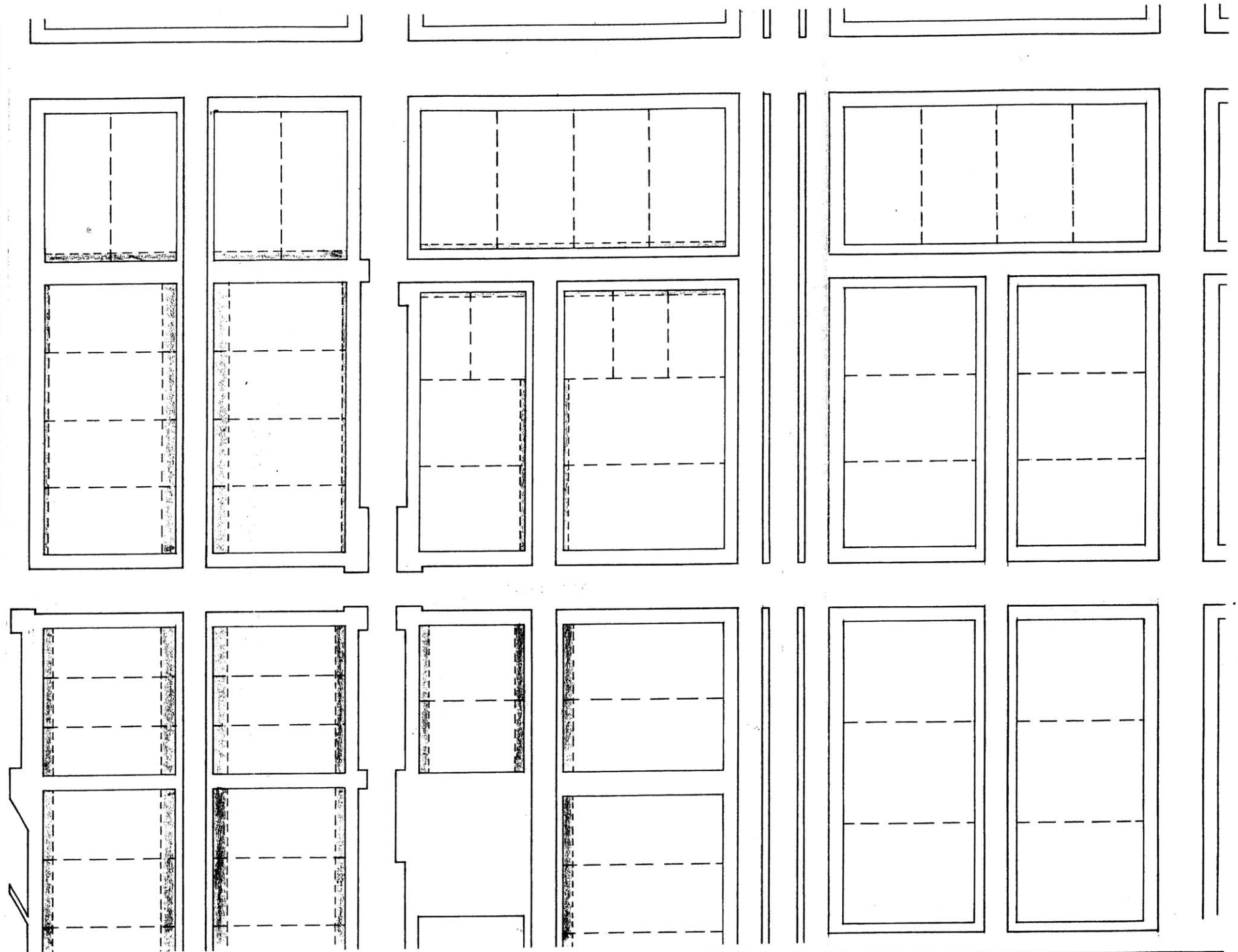
Detail showing physical implementation of street types, relationships between pedestrian access and other elements, and building edge setbacks to generate semi-public territories.
