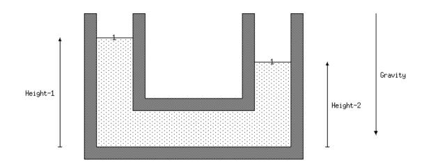
Figure 5-2: U-tube model with interpreted outputs
