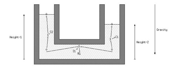
Figure 5-10: Model for U-tube with second-order behavior
