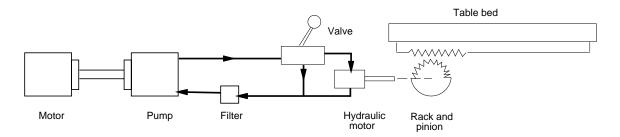
Figure 5-28: A table-bed positioning system (after [18])
