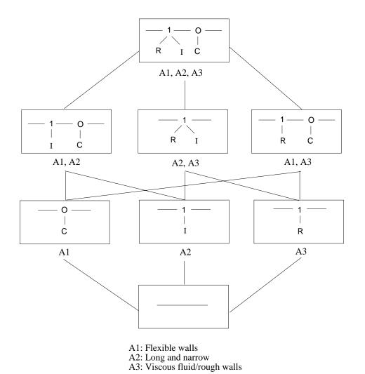
Figure 6-1: Graph of Models for a pipe
