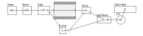
Figure 5-30: Initial bond graph for the table-bed system
