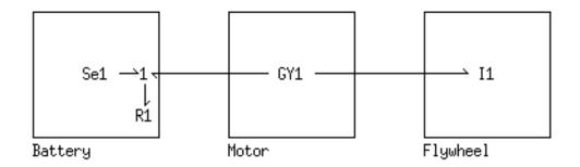
Figure 5-25: One model for the motor-flywheel system
