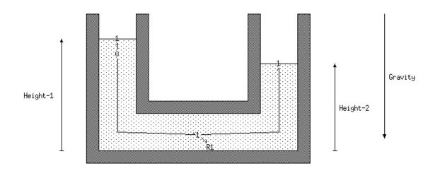
Figure 5-5: U-tube model with resistor
