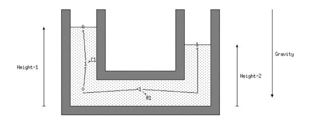
Figure 5-7: U-tube model with resistor and capacitor
