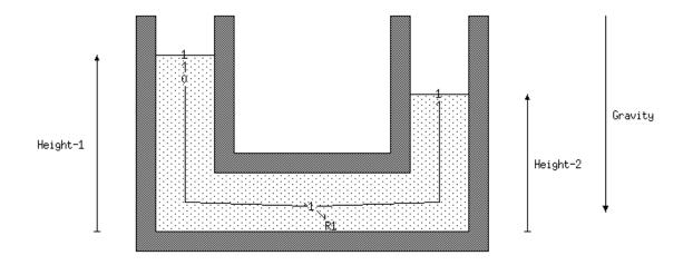
Figure 1-5: U-tube with resistance
