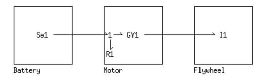
Figure 5-26: A second model for the motor-flywheel system
