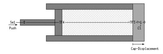
Figure 5-18: Zeroth-order piston model with capacitor
