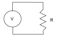
Figure 2-1: Circuit corresponding to bond graph Se—R
