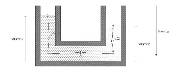
Figure 1-6: U-tube with superimposed bond graph
