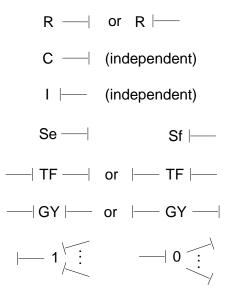
Figure 4-1: Constraints on causal strokes
