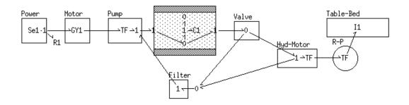
Figure 5-32: Table-bed model with resistor and fluid capacitor
