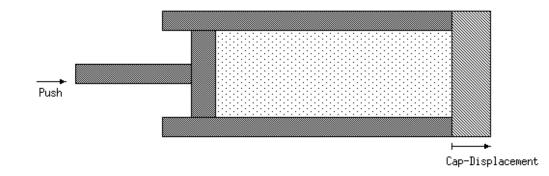
Figure 5-13: A hydraulic piston
