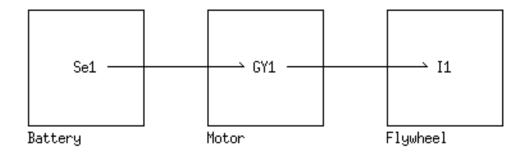
Figure 5-23: Initial model for motor-flywheel system
