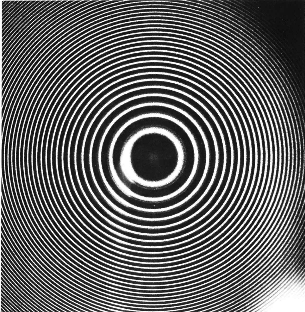
Figure 6 Fabry - Perot Plate No. 33 Four Laser Lines
