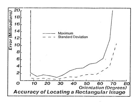
Figure 3.6: Dependency of the fitted boundary interpolation technique with image orientation for an image of a rectangle
