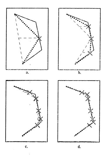
Figure 4.27: Recursive split-and-merge segmentation algorithm. The center of a line drawn between the two end points in an image of line segments is tested for being near the line segments. If it is not, the proposed line is split and the algorithm is applied to the two new lines.
