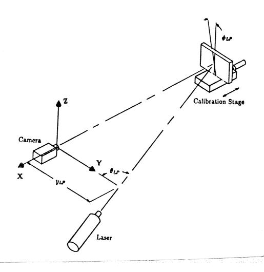
Figure 4.2: Light stripe sensor configuration.
