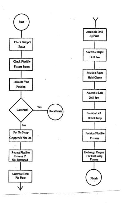
Figure 5.12: Assembly cell setup procedure.
