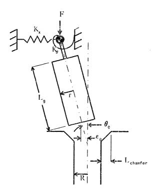
Figure 2.3: Parameters for the two-dimensional peg in hole assembly (from [201]).
