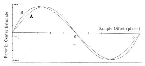
Figure 4.23: Errors in center of area estimate as a function of relative sampling position. Curve A is the numerically calculated error for 10 samples under the main part of the profile and curve B is a sinusoidal approximation to the error.
