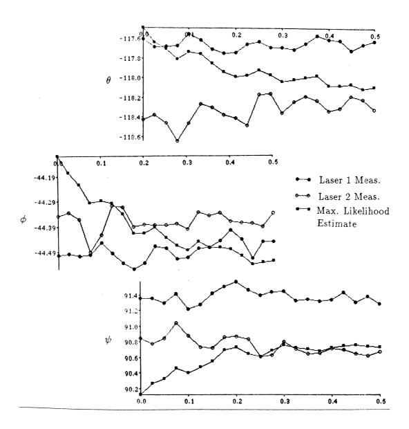
Figure 6.9: Maximum likelihood estimates of rotation angles of the test cube.
