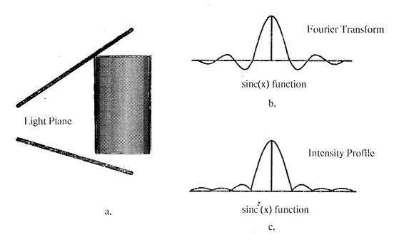
Figure 4.14: Intensity profile of a light stripe.
