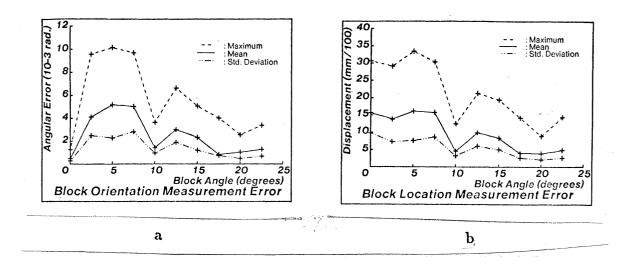
Figure 3.15: Results of the simulated corner localization tests. a. Rotational Accuracy. b. Translational Accuracy.
