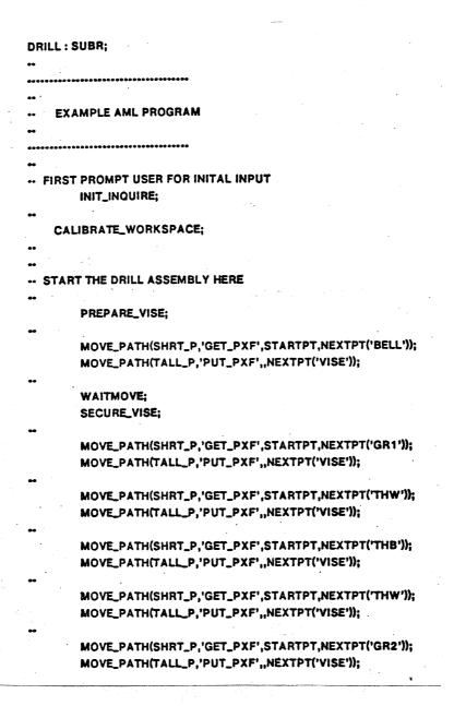
Figure 5.17: Example top level assembly program.
