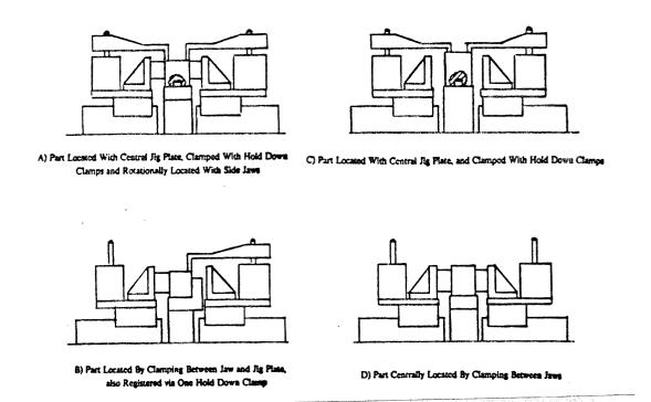
Figure 5.3: Different combinations of vise fixturing systems which may be used to constrain the base part in an assembly.
