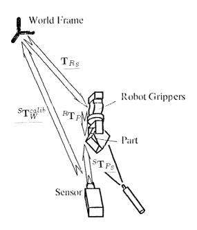
Figure 2.5: Calculation of the robot to part transformation.
