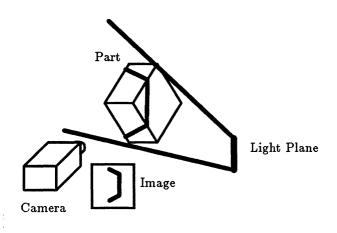
Figure 4.1: Three line segments generated by the intersection of a plane of light and the surfaces of a polyhedral feature may be sensed by a video camera and used to locate a part.
