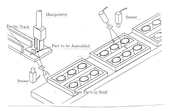
Figure 3.13: An assembly system which uses part position sensing needs no specialized fixtures. Parts are taken from a feed track by the manipulator, sensed, repositioned, then assembled. A part position sensor upline of the assembly station determines and records the position of the base parts of the assembly.
