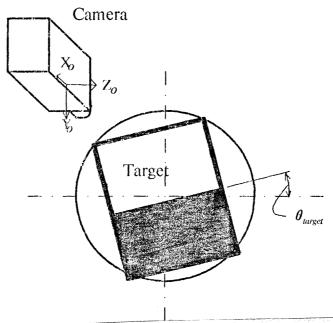
Figure 4.9: Target and camera arrangement for computer simulation and experimental tests.
