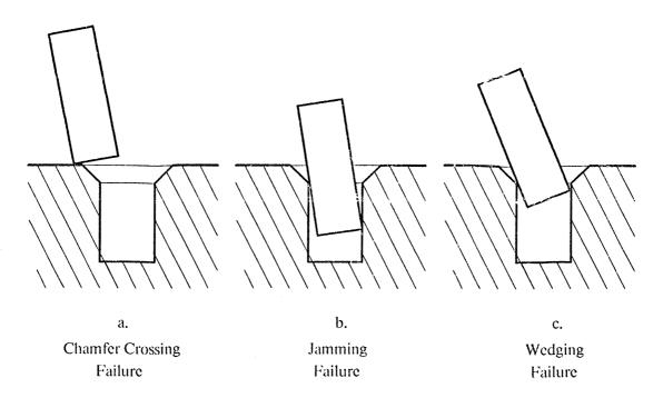
Figure 2.2: Failure modes for the peg in hole assembly. a. Initial translational alignment is not within chamfer limits. b. Jamming occurs. c. Wedging occurs.
