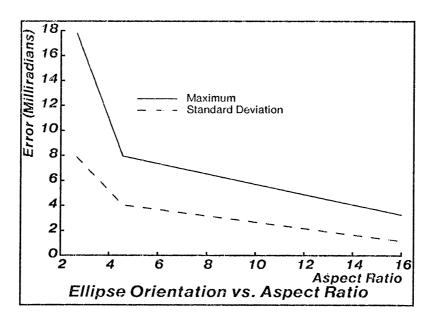
Figure 3.8: Dependence of the fitted boundary interpolation technique on the aspect ratio of an elliptical image
