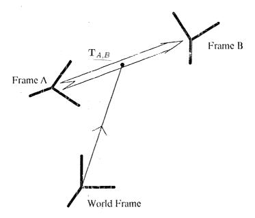
Figure 2.6: Graphical representation of a rigid transformation. The transformation shown,  $\mathbf{T}_{A,B}$ , is from frame A (six coordinates) to frame B. The extra line from the world frame to the transformation indicates that the transformation is specified with respect to this frame.
