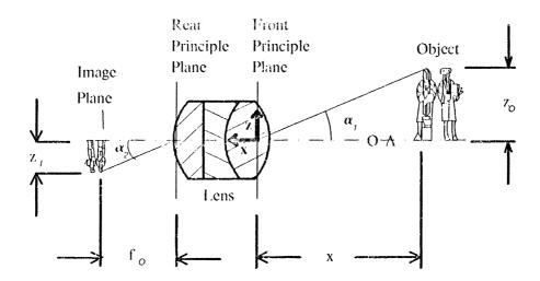
Figure 4.3: Parameters for modeling a thick lens.
