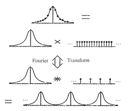
Figure 4.18: Fourier transform of a sampled Gaussian.
