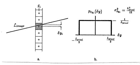
Figure 4.6: Probabilistic location of points on a line. a. Intersection of a column of pixels with a line in the range  $\theta \in \left[-\frac{\pi}{4}, \frac{\pi}{4}\right]$ . b. Probability density function for the location of the y coordinate of  $\mathcal{L}_{image}$  measured from the center of the illuminated pixel.
