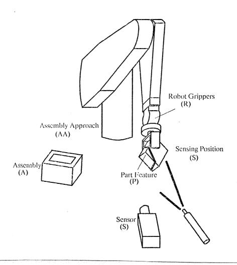
Figure 2.4: Sensor-driven assembly system.
