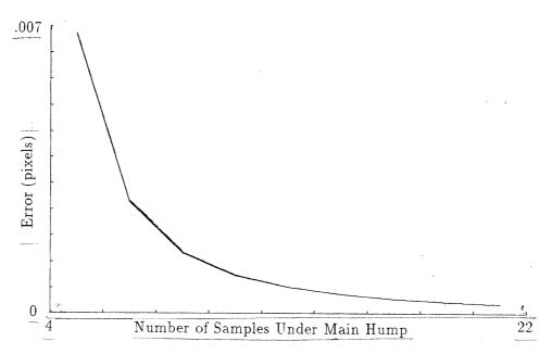
Figure 4.24: Standard deviation of errors due to sample offsets of a  $sinc^2(x)$  shaped intensity profile as a function of the number of samples.
