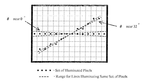
Figure 4.11: Range of motions of lines before change in state of sensor occurs.
