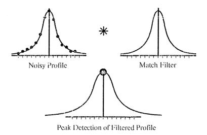
Figure 4.25: The match-filter and peak detection procedure for determining the location of the peak of an intensity profile entails filtering the image with a match filter then performing a peak detection in the filtered profile.
