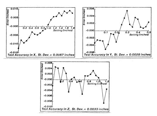
Figure 6.12: Results from the PUMA local accuracy tests. Robot motion in the x, y, and z directions are along the abscissas and measured position deviations are along the ordinates. The standard deviations listed correspond to errors over the full range of motion indicated.
