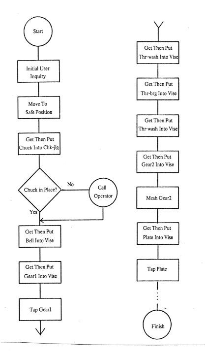
Figure 5.18: Drill assembly procedure.
