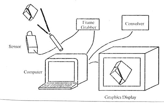
Figure 4.26: Sensing and image processing system components.
