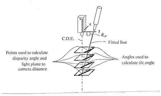
Figure 6.5: Method for determining the disparity angle, tilt angle, and light plane to camera distance.
