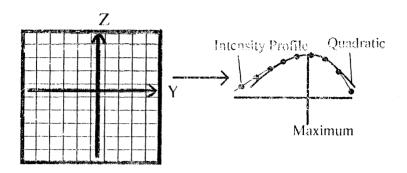
Figure 4.28: Coordinates used for the line fitting algorithm.
