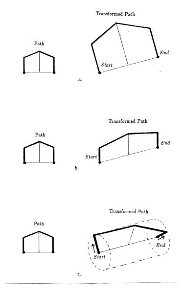
Figure 5.11: path transforms. a. Spatial path transform. b. Planar path transform. c. Cylindrical path transform.
