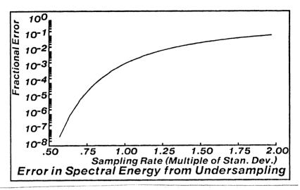
Figure 4.19: Fraction of energy lost in the frequency domain due to undersampling a Gaussian.
