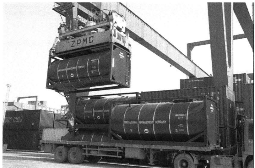
Figure 5: Container Tanks with a Quay Crane, Truck & Chassis at Port (Alibaba.com, 2011)
