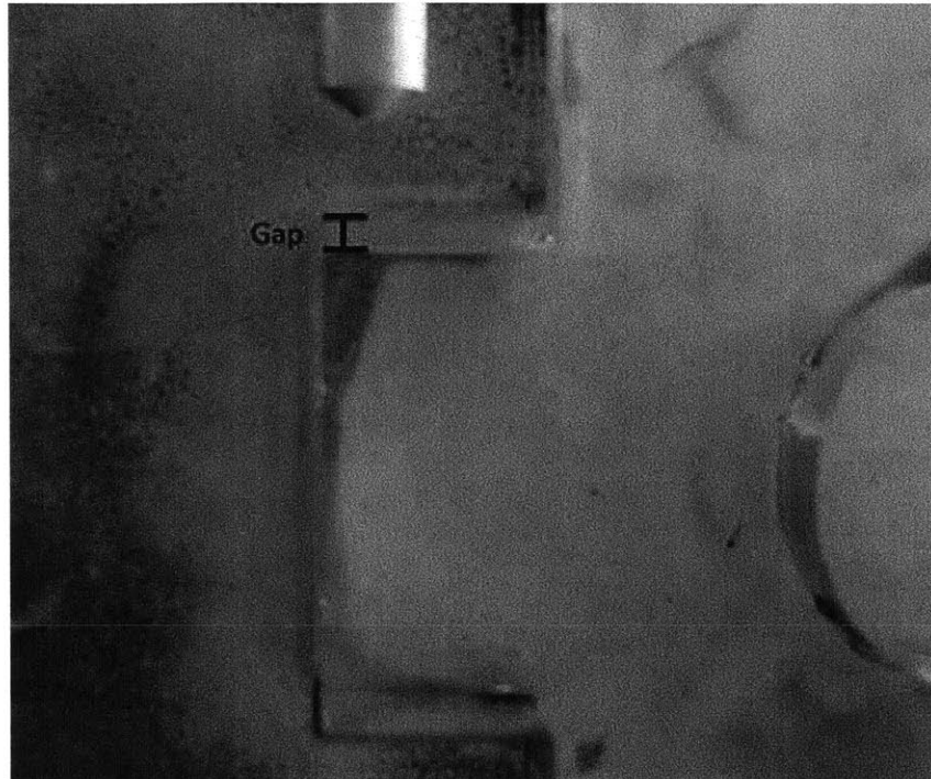
Figure 33: Gaps in the parts as a result of not taking the laser cutting width into account.
