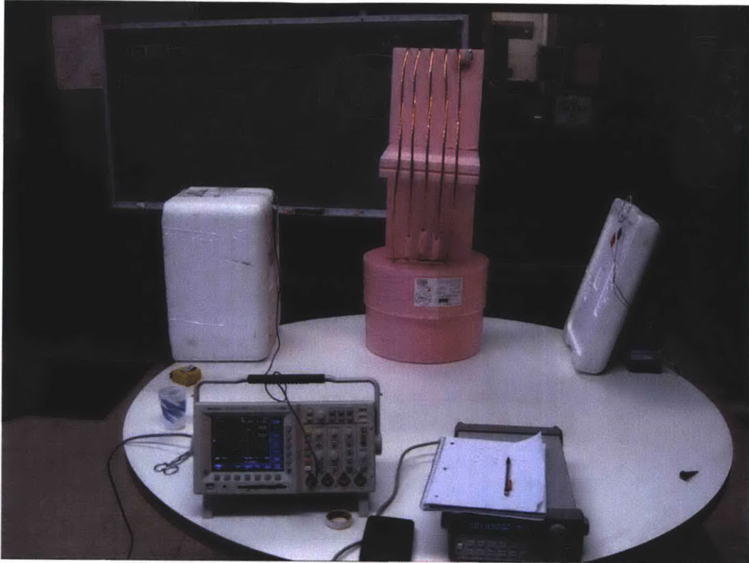
Figure 3-2: Experimental setup for measuring the resonant frequency and quality factor Q of a resonator. The self-resonant coil (center) is excited by a coil connected to a CW source (right), and the amplitude of its excitation is picked up by coil connected to an oscilloscope (left). The quality factor is found from the FWHM of the measured amplitude as the frequency of the CW source is swept.
