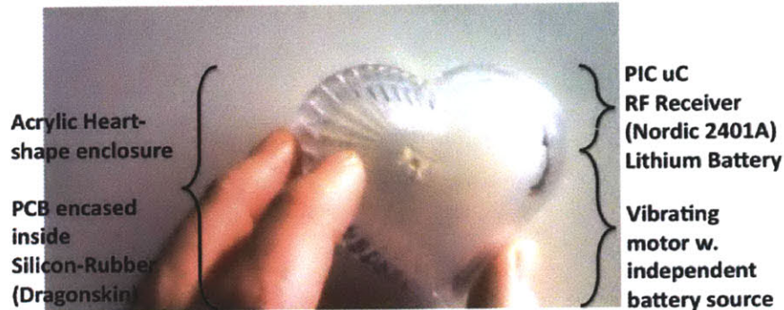
Figure 4-1. The MiniHeart is a hand-held heart rate indicator that wirelessly receives beat-to-beat heart rate signals and then represents them as pulsing LED lights and vibrations.
