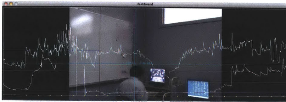
Figure 4-5. Interactive Physioboard collects and processes two skin conductance inputs (the participant's and the occupational therapist's). The user can move the mouse along the x-axis to retrieve images dynamically at the specific time in an interactive way.
