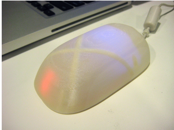
Button-less prototype with SparkFun breakout board and parts printed on the Dimension.
