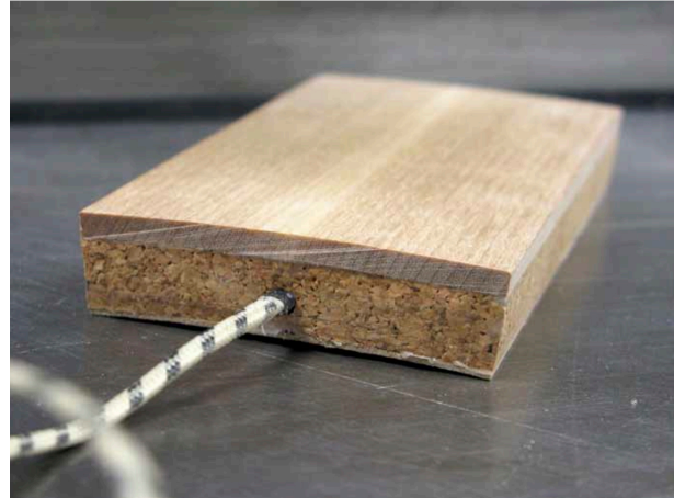
Force sensor in cork and wood [Cottam 2009].
