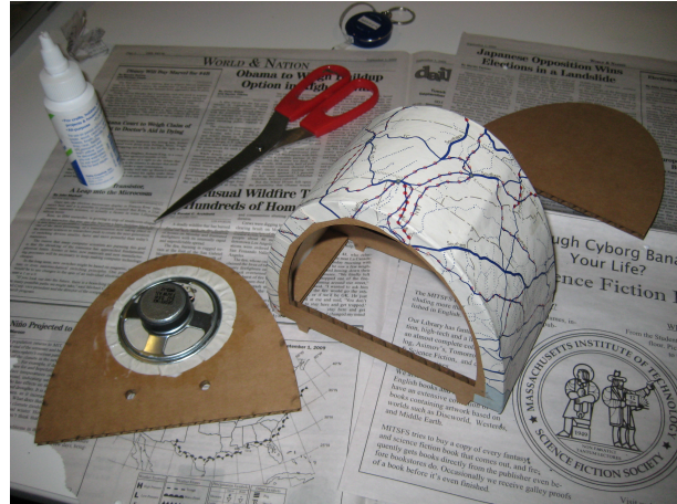
Cardboard and paper prototype of the Fab FM structure. (photo by Dana Gordon)
