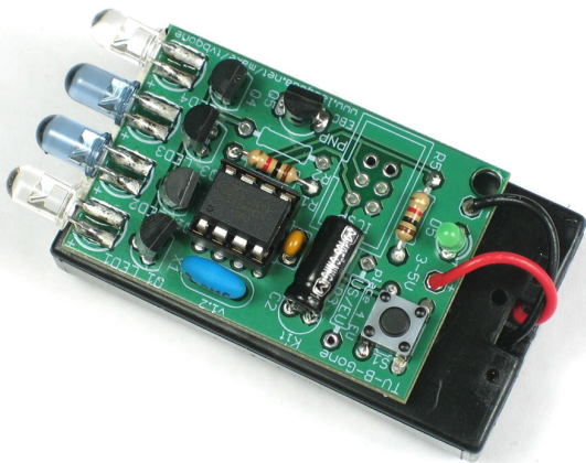
Assembled TV-B-Gone kit from Adafruit Industries.
