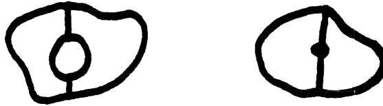
Figure 24. In an N-space structure, the intersection of any set of cells must be exactly one cell or empty. Thus, two cells cannot touch along two disconnected faces, as shown on the left. Nor can the common face of two cells be split into several cells, as shown on the right.
