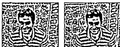
Figure 7. A stereo pair contains two images of the same scene, taken from slightly different viewpoints. This figure shows the edge finder output for such a pair of images.
