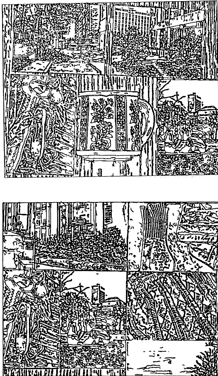
Figure 6. Phantom edge finder results for the two images in Figure 4, using noise threshold 60.
