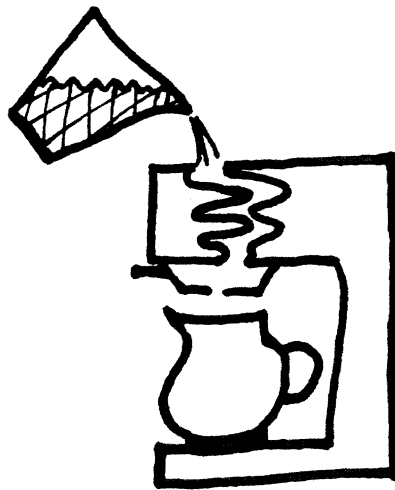
Figure 8. If water is poured into the top of a coffee maker, it will eventually flow out the bottom, because there is a tube connecting the water input and the water output.
