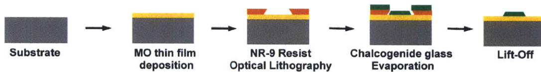
Fig. 2-3 A schematic plot of the fabrication process using optical lithography and lift-off methods
