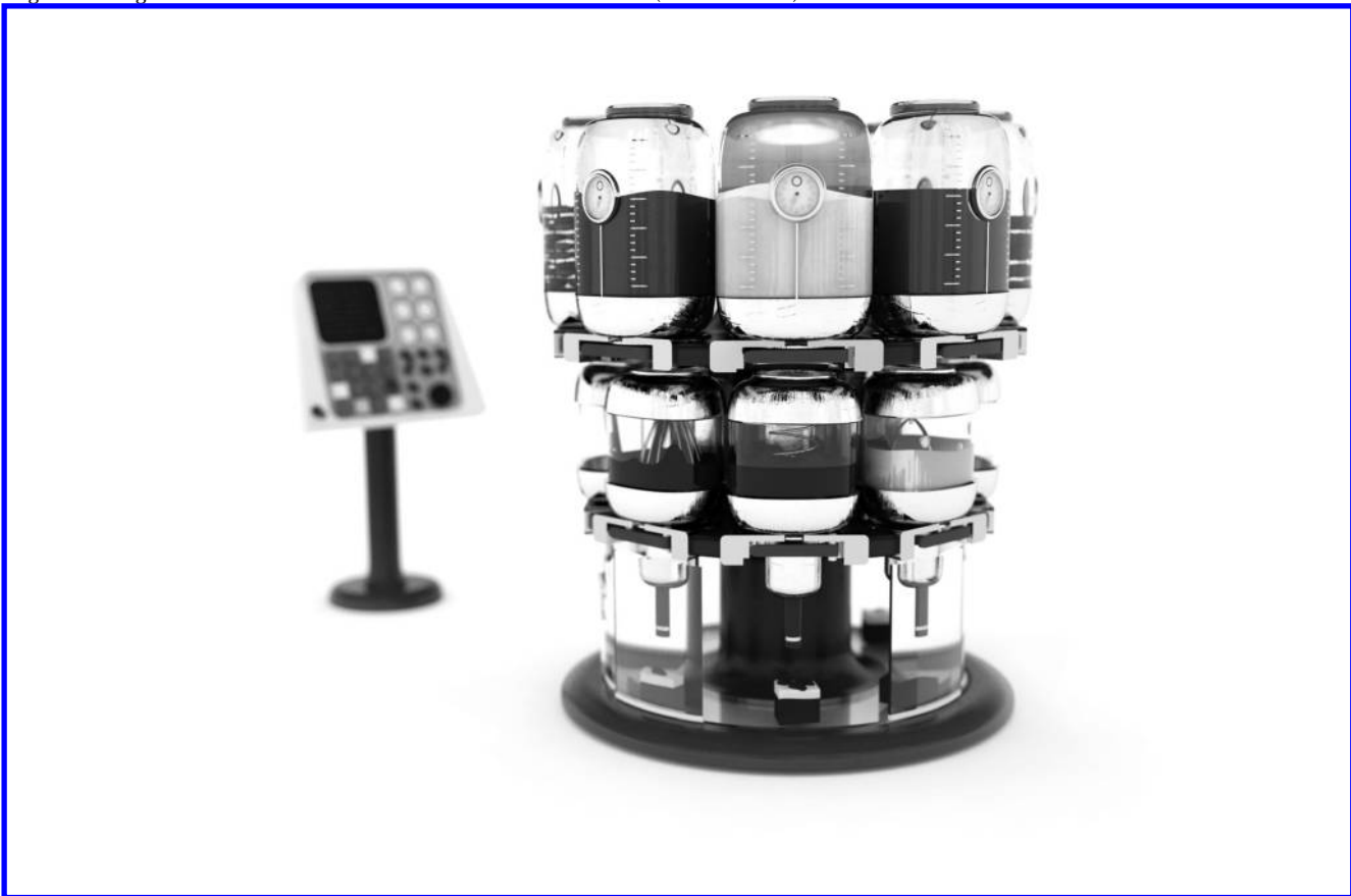
Fig. 2. The ingredients-combination machine—The Virtuoso Mixer. (© Amit Zoran)
