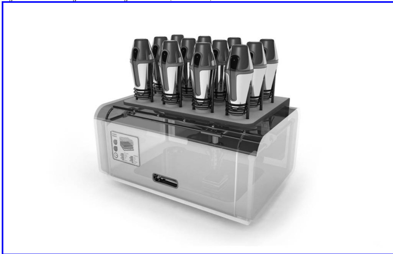
Fig. 3. The food-modeling machine—the Digital Fabricator. (© Amit Zoran)
