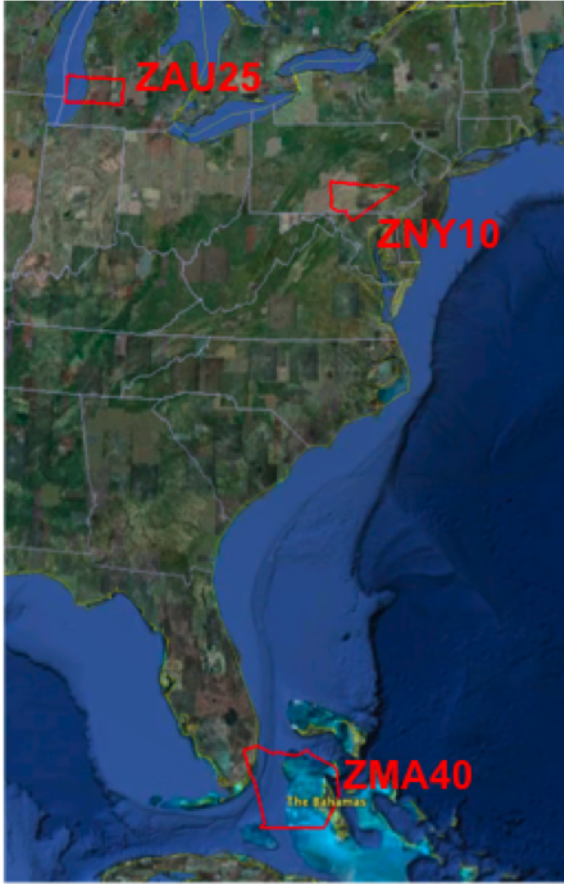
Figure 5-3: New York 10 (ZNY10), Chicago 25 (ZAU25) and Miami 40 (ZMA40) were selected for the communication analysis. Among the ATC facilities for which public voice communication was available, these sectors satisfied the constraints of (1) being located in the higher stratum of the NAS (ceiling above FL240); and (2) presenting intermediate level of communications
