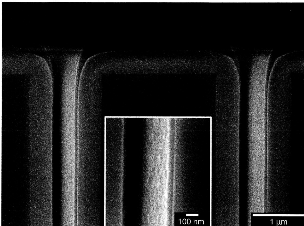
Figure 4-4 SEM micrograph of the nanochannels coated with a 90 bilayer \text{TiO}_2/\text{PVS} multilayer after calcination. Inset: highly magnified view showing a nanoporous titania film on a nanochannel wall. Courtesy of Dr. Jun Young Kim.
