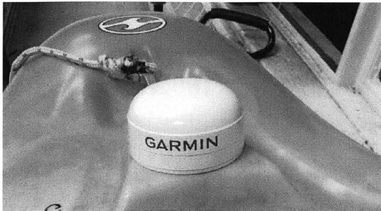
Figure 2-13: Garmin GPS installed on kayak
